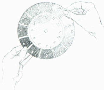
Fig. 6-5. Use the outer punched holes to determine the value level.
